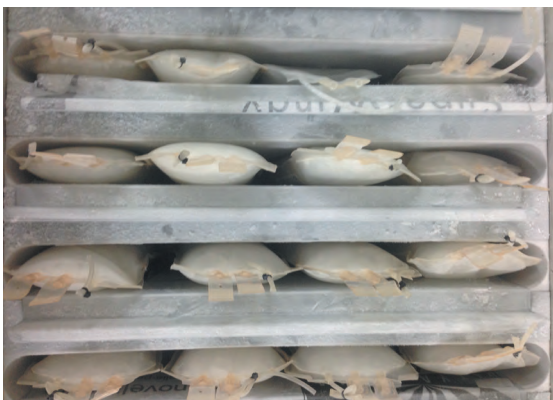
Internal case of the rapid freezer with standard 1000 ml. bags in freezing
